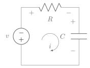
Figure 8: Converting Pulse Width Modulated (PWM) signal to its DC value. The capacitor charges to the mean value of the PWM. For 255 this will be the half of the supply voltage, i.e., will yield 2.5V.
